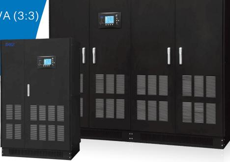
EA890 series UPS 80  $\sim$  500 kVA provide maximum protection and power quality for mission critical loads, including data centers, industrial processes, telecommunications, security and electro-medical systems. It is an on-line double conversion UPS with IGBT based 3-level PWM rectifier technology, featured with high input power factor (> 0.99), low THDi, high efficiency and built-in output isolation transformer.
